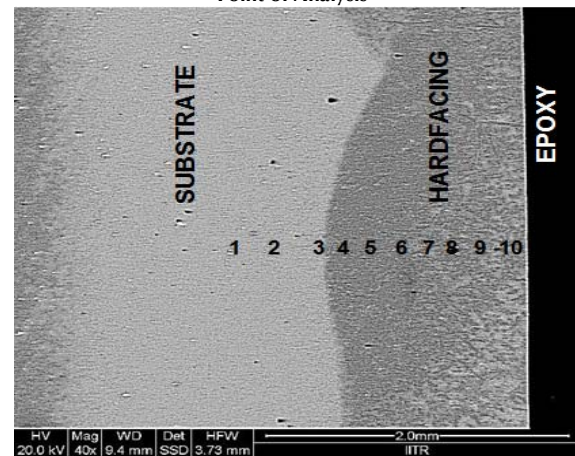
Fig. 3: Morphology and Elemental Composition at Different Points along the Cross-section of Hardfacing Overlay (HF)
